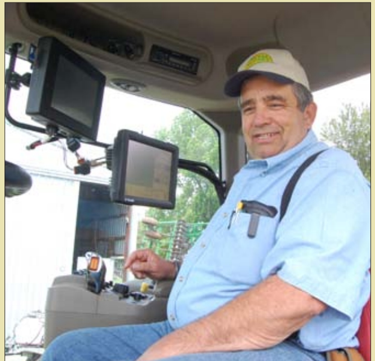
UPLOAD QUEUE: Once Doug Chaffer finishes a field, his FmX unit queues the data for the next time he's within range of his wireless network.
